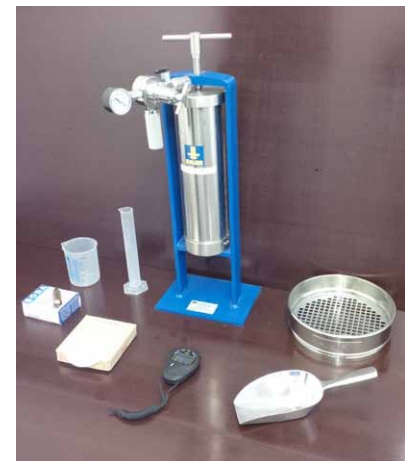
FIGURE A.8: Test set-up to determine water filtrated from pressurized fresh concrete (Bauer)
